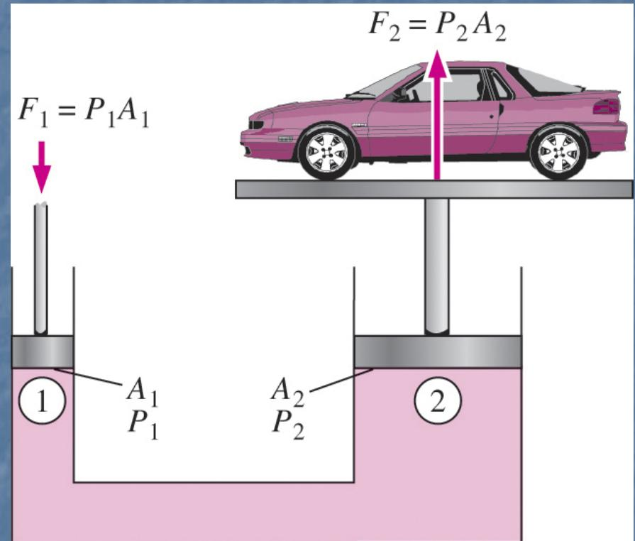
Lifting of a large weight by a small force by the application of Pascal's law.
